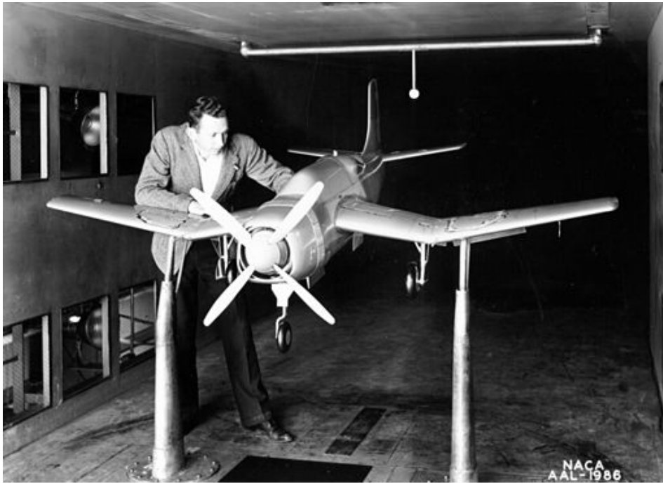
Figure 2.23 – An Example of a High Fidelity Prototype of a Plane, the Douglas SB2D ‘Destroyer’ Being Tested in a Wind Tunnel (NACA, 1942)
