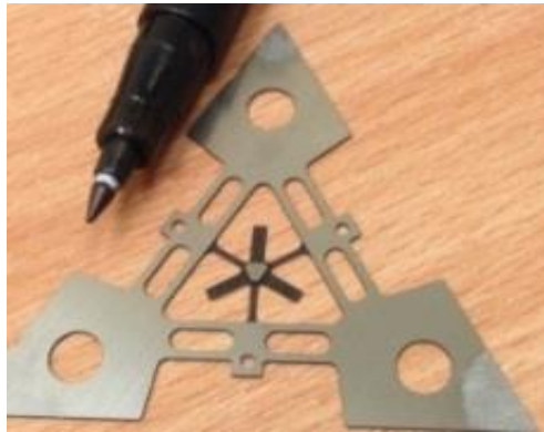
Fig. 5. Photograph of the middle layer of the smart suspension structure, the thin sections of spring beams and paddles appear to be darker in colour due to the chemical etching process.
