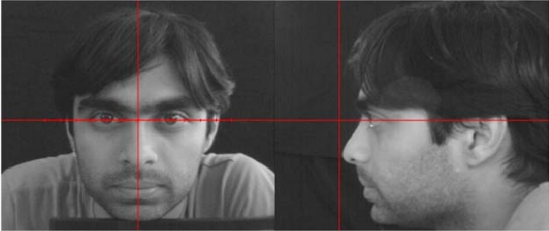
Figure 2: Datum cursors for the initial camera set-up. Left, frontal view and right, profile view.
