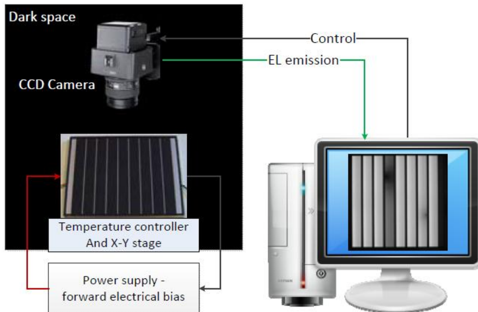
Figure 2.19. Schematic of an EL system. The EL measurements are carried out in the dark. NIR Light emission from the radiative recombination is excited by the external electrical bias applied at the terminals of a PV cell. This schematic shows the basic experimental setup of imaging characterisation systems.
