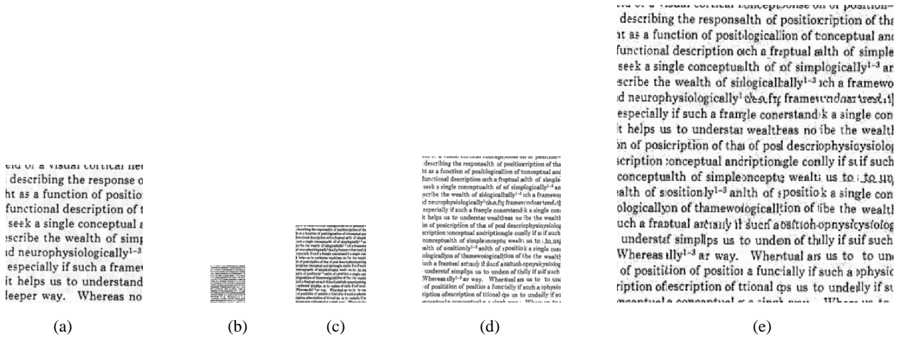
Figure 6: Input texture and output texture constructed using coefficients at different levels (a) Input texture ( I_{sample} ). Output texture constructed, (b) using only low-resolution details of the third level ( I_{oa2} ) (c) using all 3 rd level details ( I_{oa1} ) (d) using 3 rd and 2 nd level details ( I_{oa0} ) (e) using all details of all levels ( I_{output} )
