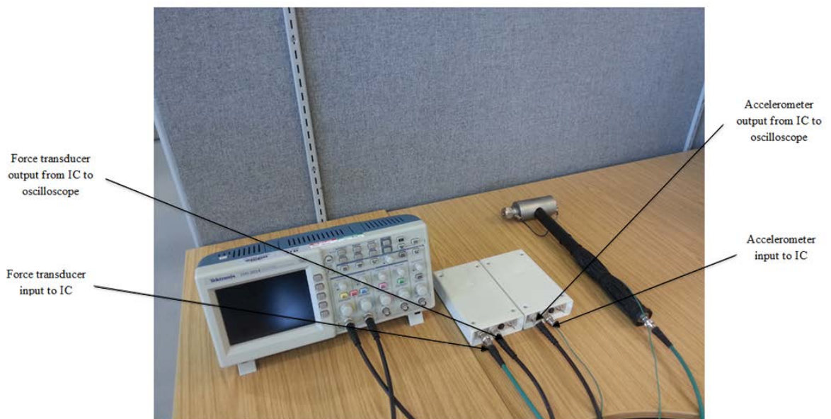
Fig 41 - Instrumented hammer set-up
