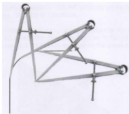
Figure 2.3.8 – Scribing at an angle
