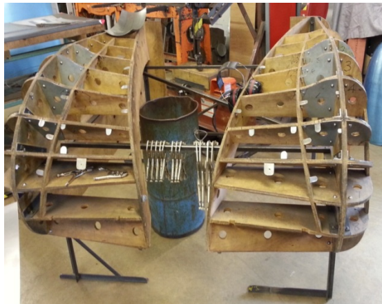
Figure i – Jig of XK Jaguar Body
