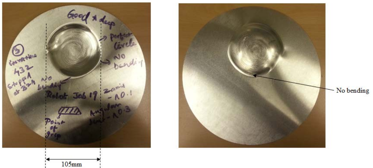
Fig 92 - Results based on skewing sheet metal perpendicular to the hammer's centre
