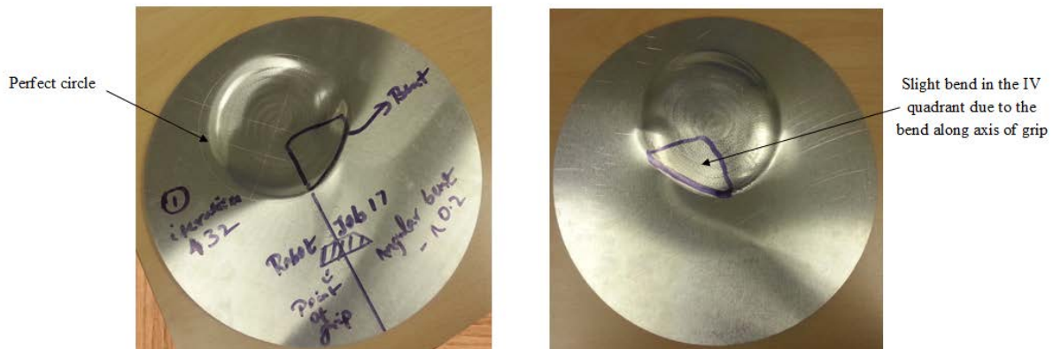
Fig 90 - Results of minimising the step angle to 10 degrees
