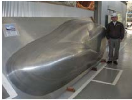
An example application of ISF – a 1/8 scale model of the front section of a Shinkansen (Bullet Train) made by Amino in Japan.
