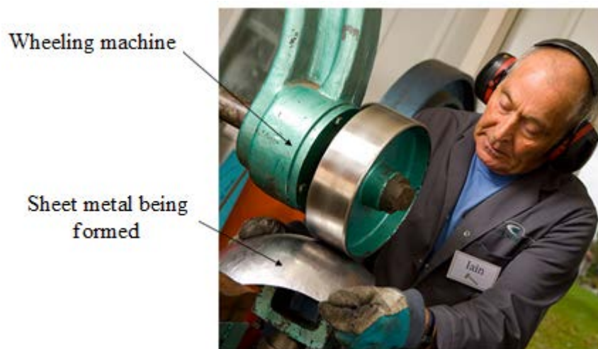
Fig 8 - Using a wheeling machine for contour finish
