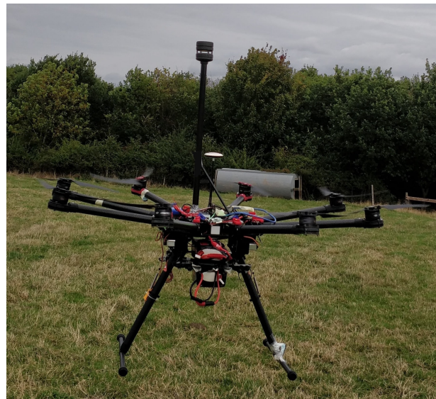
Fig. 6: S1000 with FT742 ultrasonic windspeed sensor mounted out of rotor wash
