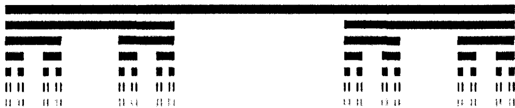
Figure 2.11: The initiator and the first six steps in the construction of the Cantor Set.
