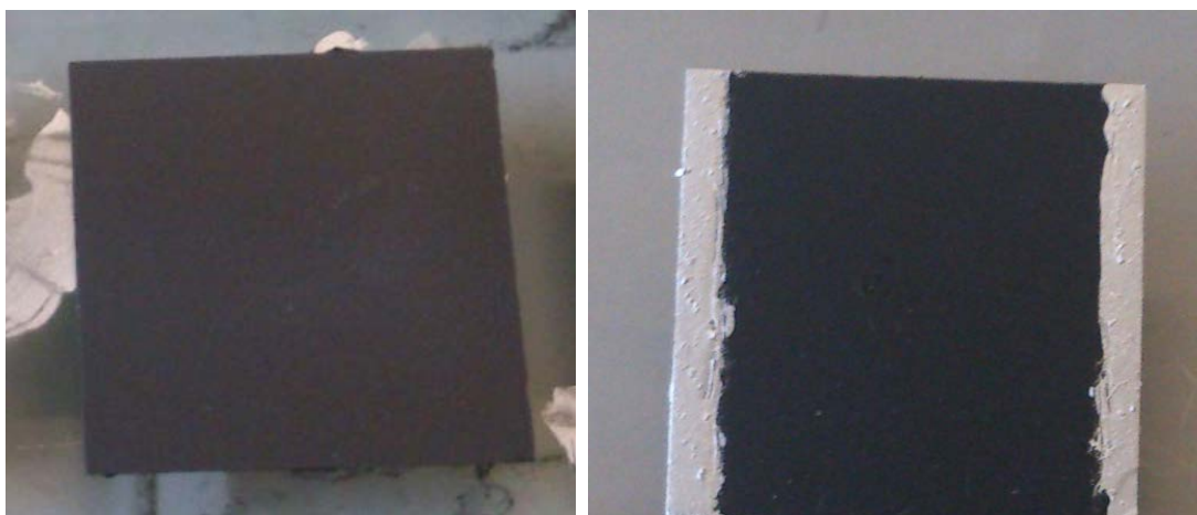
Figure 2-4: Digital picture of the sample of GO/MWCNT at final stage after drying and before measurements.
