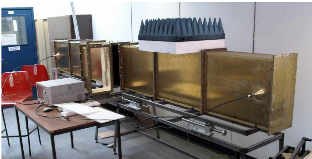
Figure 5.12: 0.35-0.53 GHz waveguide measurement facility at Sheffield University, UK
