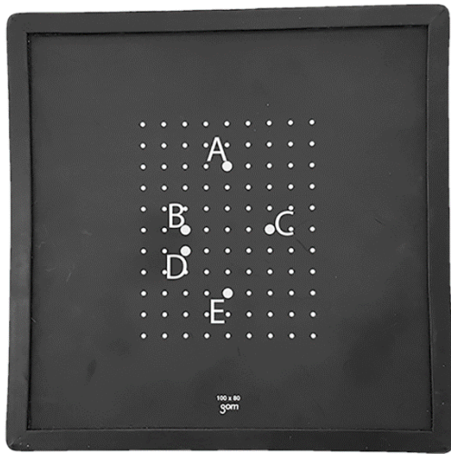
Figure 7: The GOM calibration board used for the point tracking accuracy investigation. The points used in this analysis are marked A – E.
