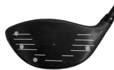
Figure 5: Foresight HMT markers placed on the driver clubface
