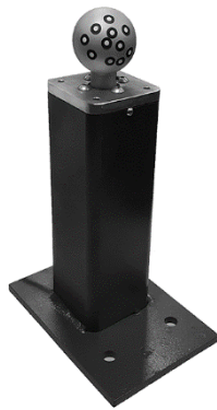
Figure 8: The custom-built, GOM marked spinning device used to assess the GOM spin rate calculations.
