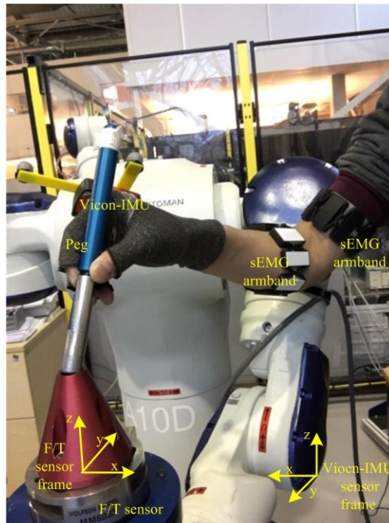
Figure 5-1 Experiment setup for PiH. The operator is wearing two sEMG armbands to record the muscle activations. A Vicon-IMU system is installed on the hand for tracking hand motions. An F/T sensor is statically installed to record the reference contact force signal.
