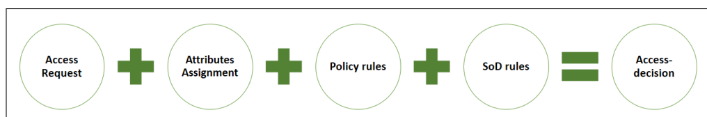
Figure 6.5: ABAC sh processing stages
