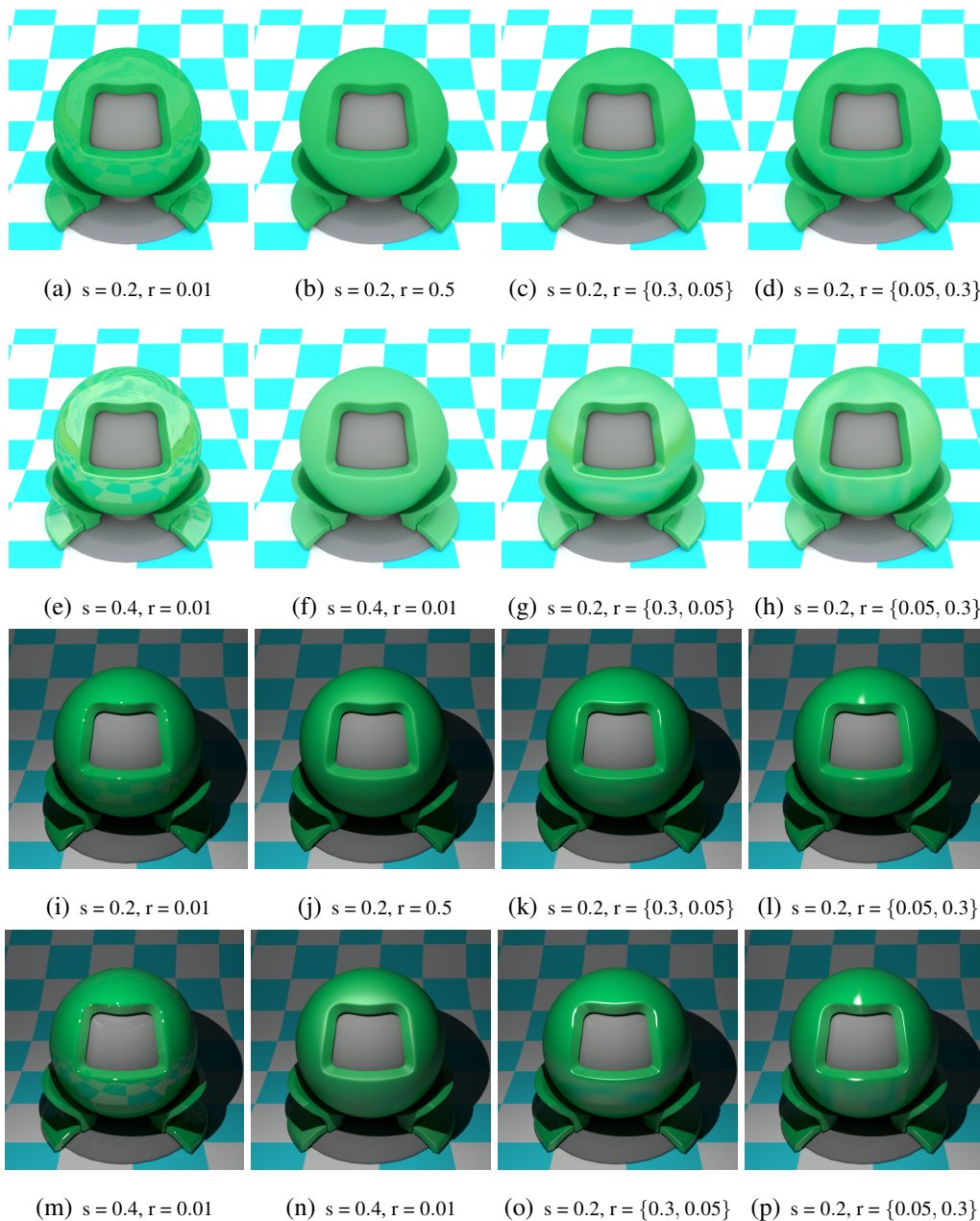
Figure 2.6: Energy conserving Ward model variant [2]. The first two columns refer to an isotropic material, whereas the last two columns refer to an anisotropic material. The top two rows reports a sequence of renderings under environment map lighting. The bottom two rows show the same sequence under a point light illumination. The parameters used are reported in brackets: the first value ( s ) refers to the specular reflectance, the second value ( r ) to the isotropic roughness, or in case of anisotropic material the second value refers to the roughness in the tangent direction, the second one to the bitangent direction.
