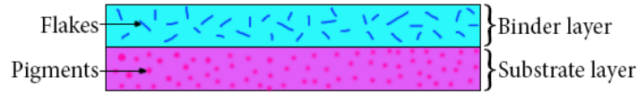
Figure 2.9: The bi-layered model by Ershov et al. [3]. The substrate layer is a solid paint film where the reflectance is Lambertian and the transparent binder layer contains embedded flakes.
