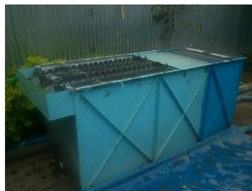
Photograph 2. Modified IPS prototype with hydraulic flocculator extension and overflow launders
