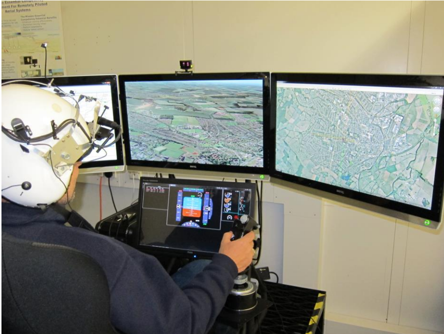
Figure 3.22 - Top left - Questionnaire Screen, Top Middle - Main Flight Visual, Top Right - Google Earth with flight path and rough object location, Bottom - Flight Instrumentation & final configuration
