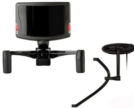
Figure 3.24- TrackIR with track clip pro by Naturalpoint ( http://www.vrconcepts.co.nz/ )
