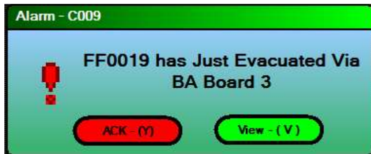
Alarm Displaying BA Wearer Evacuation via a Different BA Board for BAECOs (Figure A5.2.39)
