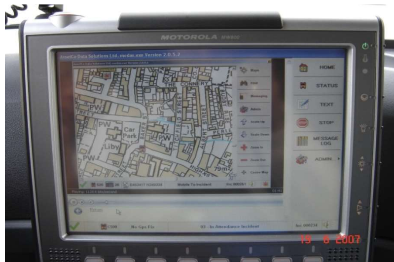
Figure 5.7: Mobile Data Terminal Installed inside the Fire Tenders
