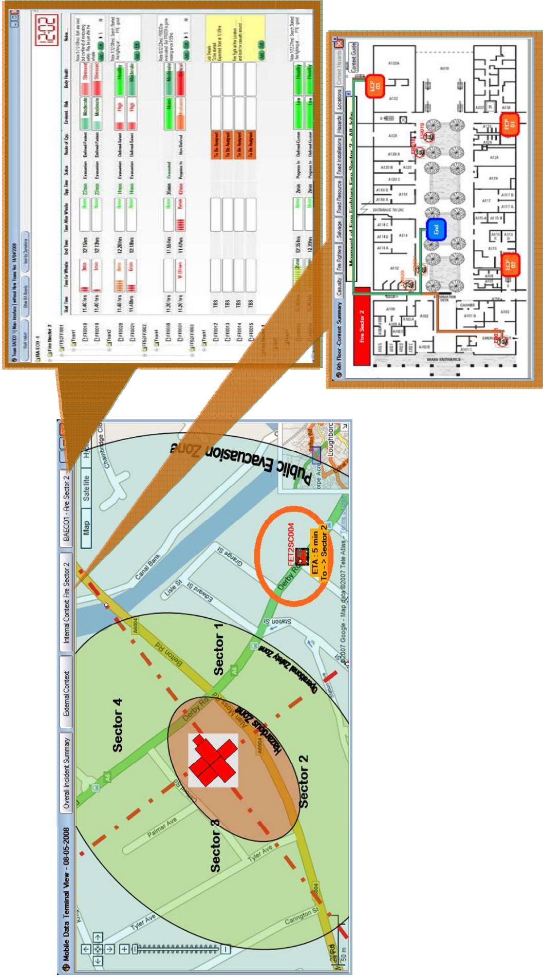
Figure 5.40: Interface Supporting Fire Fighters on the Move
