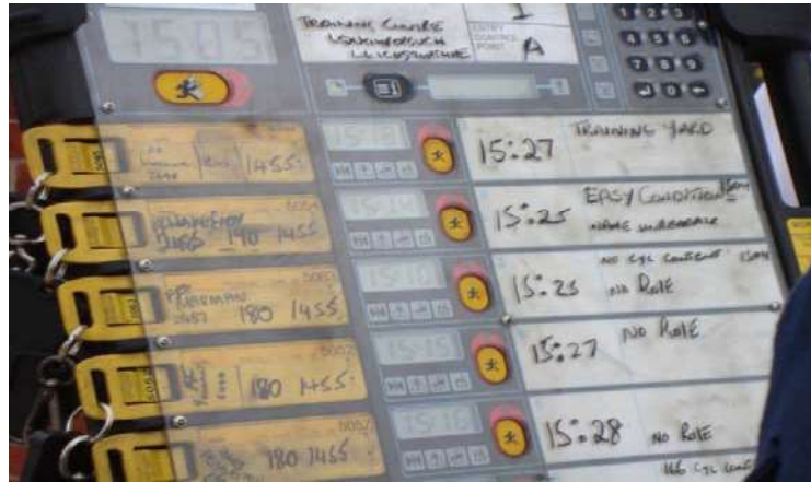
Figure 5.3: DragerMAN PSS Merlin Electronic BA Board Used by the Leicestershire Fire and Rescue
