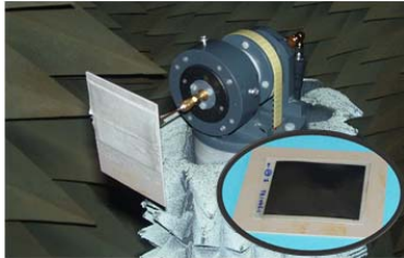
Fig. 5. The inkjet printed patch antenna in the anechoic chamber and inset the patch antenna before the connection was made
