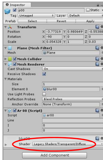
Figure 6.4: Assigning transparent shader to objects having transparent textures
