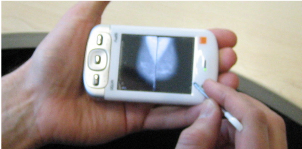
Figure 4-1. The PDA used to display mammograms in part 1 of the study
