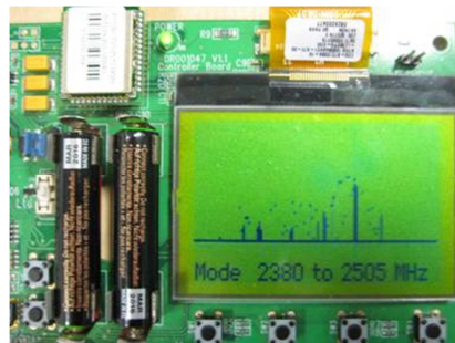
Figure 5.13 802.11b traffic 10 packet/second, 802.15.4 sampling period 1024 \mu s
