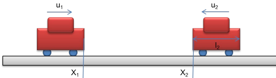
Figure 2.5 Calculation of TTC for rear-end collision type
