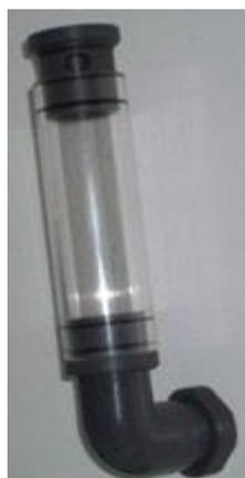
**(c) Nozzle that introduces moisture inside the chamber**
