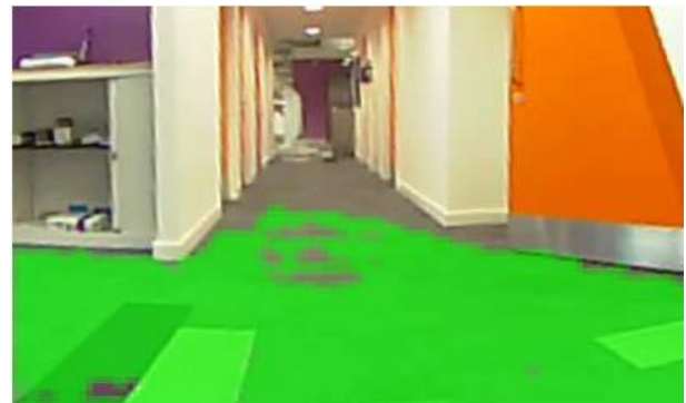
Fig. 5. Free Space Detection: Initial results: Green color indicates areas that are void of obstacles
