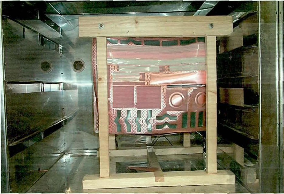
Figure 4.2 Test coupon panel in Temperature Cycling Chamber
