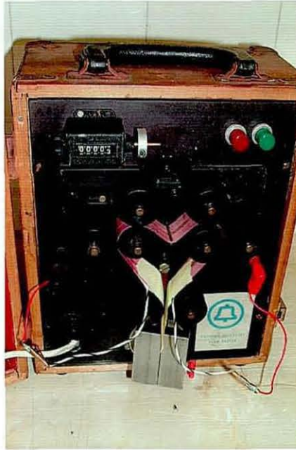
Figure 3.5 FPC Undergoing Flexural Fatigue Life Test Using a Universal Flex Tester
