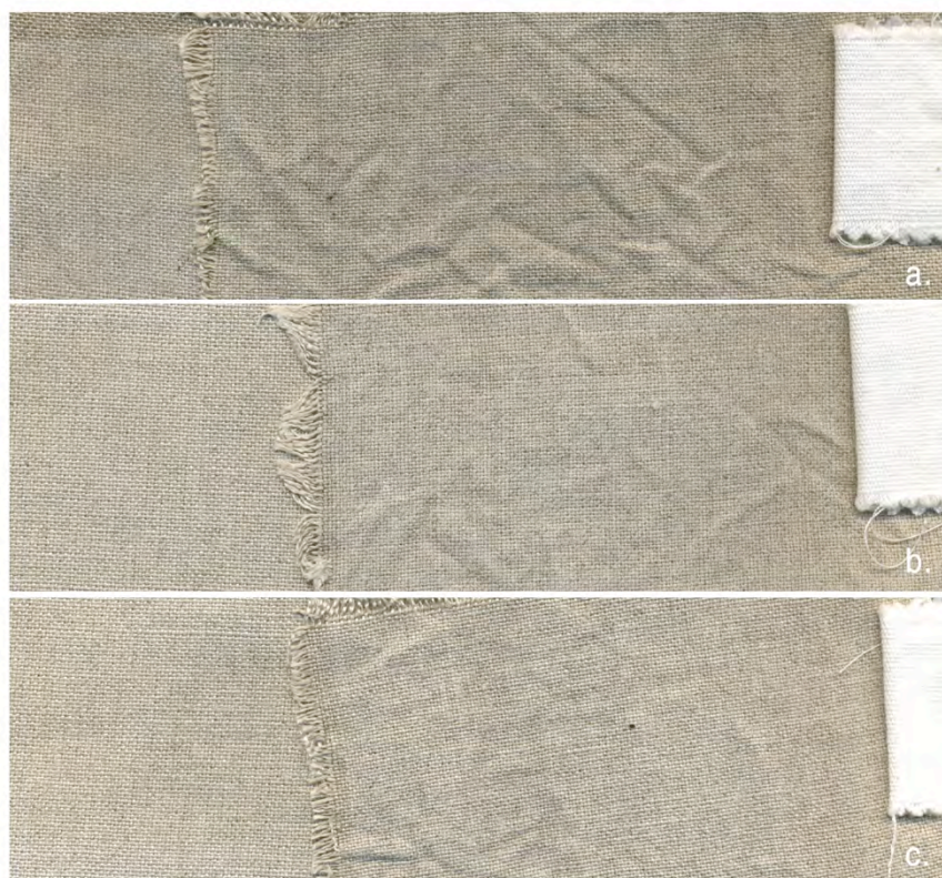
Figure 8.5 Colour fastness to washing: Laser faded linen at energy densities of a) 0\text{J}/\text{cm}^2 , b) 2.9\text{J}/\text{cm}^2 , c) 3.4\text{J}/\text{cm}^2
