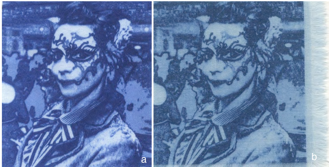
Figure 6.28 Photographic Images Peri-Dyed on a) Polyester, b) Wool.
