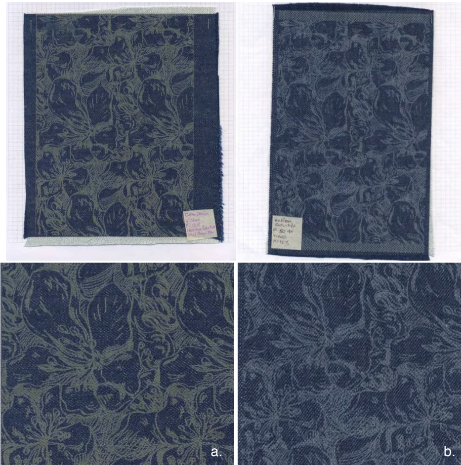
Figure 4.27 Laser fading experiment: Laser Resolution ( sample 3 ): a) 300dpi; b) 85dpi
