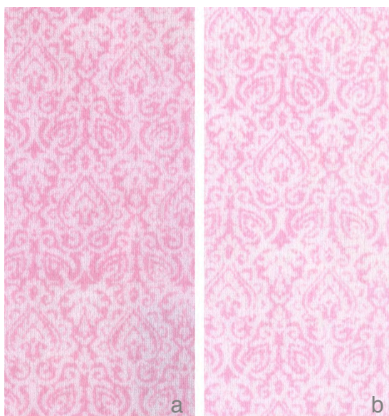
Figure 6.16 Peri-dyed Sample a) Water rinse, b) UPL rinse.
