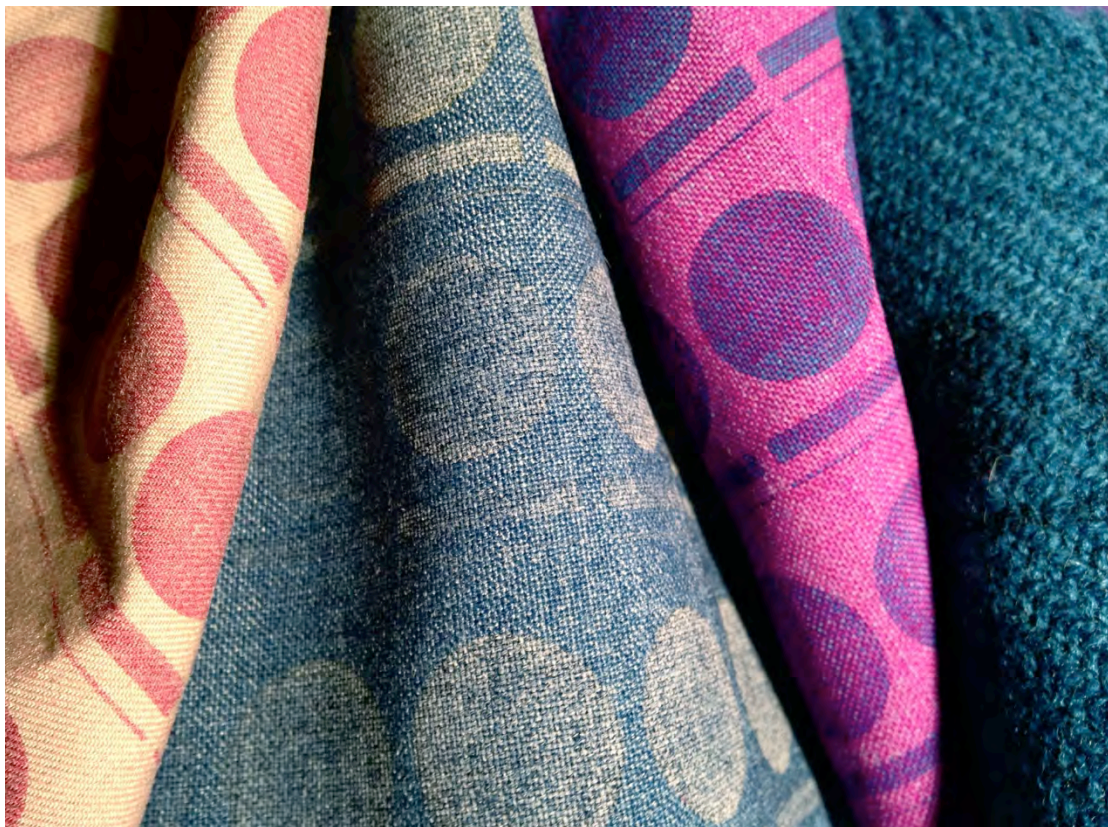
Figure 5.38 Laser Patterned 55/45 Poly/Wool design samples dyed with contrasting disperse and acid dye colours.
