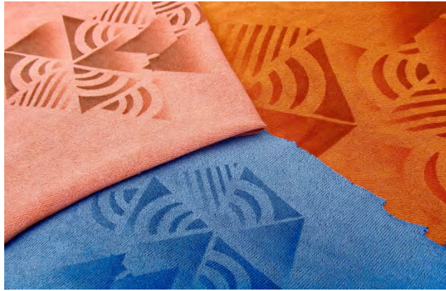
Figure 6.30 Peri-Dyeing on a Pre-Coloured Ground
