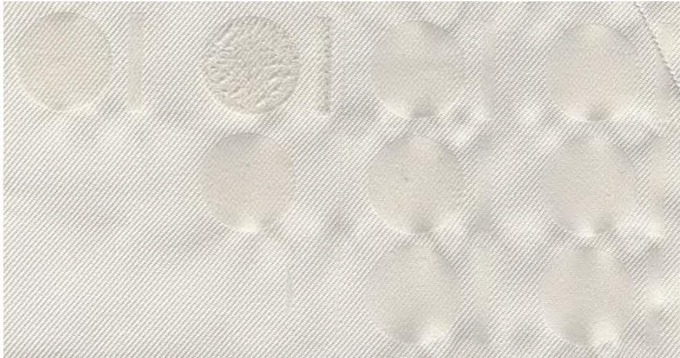
Figure 4.30 Altered surface qualities of polyester textile after laser irradiation ( sample 10 )
