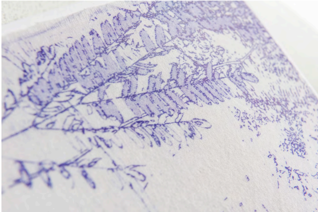
Figure 10.4 Laser peri-dyeing technique allows intricate targeted surface design of textile substrates.
