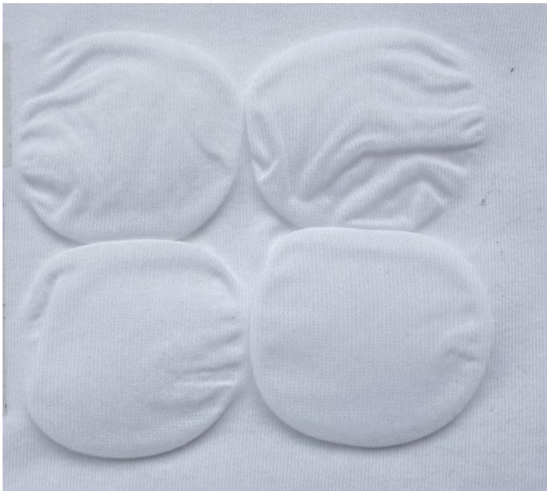
Figure 7.6 Laser Moulded Circles processed using Tapestry Frame
