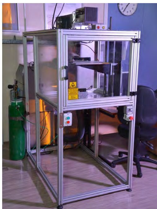
Figure 4.1 Synrad CO 2 Laser Marker Used in this Research
