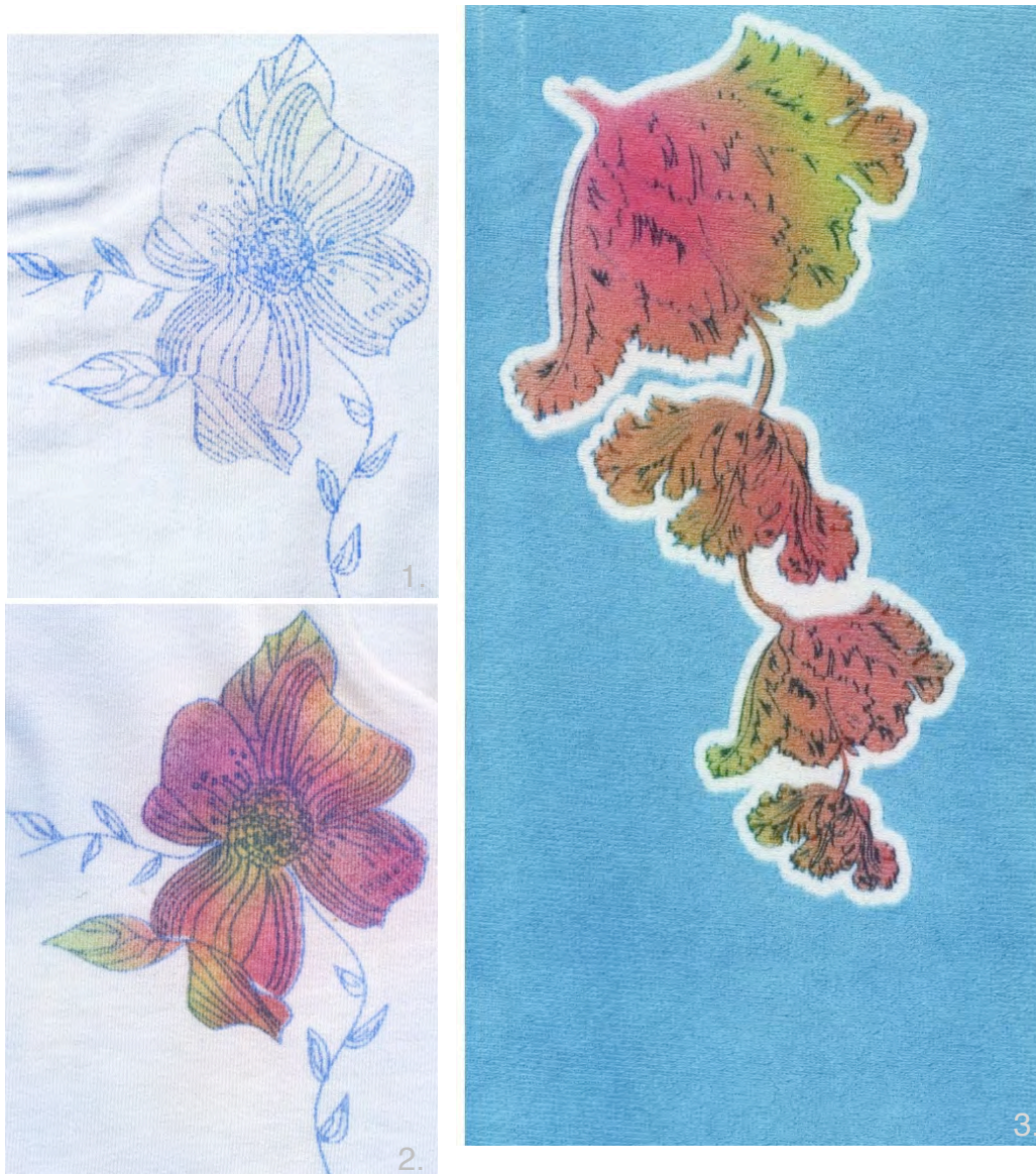
Figure 6.36 Peri-Dyed Sample: Layer 1) Blue dye applied followed by laser irradiation of linear flower outlines and background, Layer 2) Red and Yellow dye applied and allowed to mix followed by laser irradiation of inner flower, 3) Alternate design example
