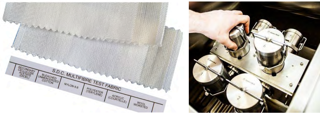
Figure 4.10 a) Multi Fibre Strip b) Wash Fastness Testing Carried out in Controlled Conditions (SDC, 2003)
