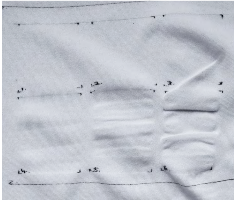
Figure 7.7 Laser Moulding Increasing Fabric Extension using Tapestry Frame
