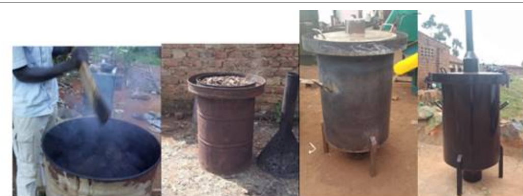
Figure 3. Metallic drums showing the modifications
