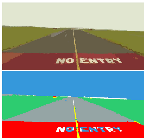
Fig. 6 Discretised HSV colour image and subsequent Bayesian network colour classifier output
