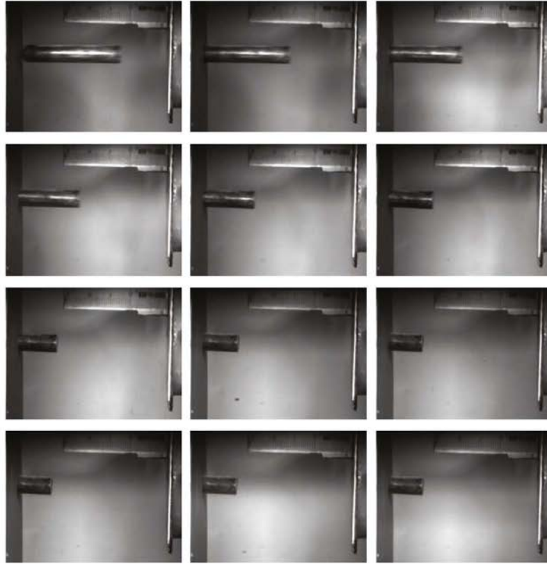
Fig. 7. High-speed sequence of penetration event at 40.84 m/s. Images taken at 5468 fps.
