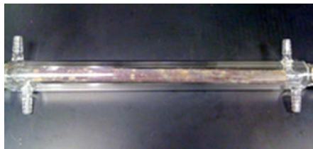
Figure 6. Layer crystallization apparatus used in the experiments. 18x8mm (300 x 300 DPI)
