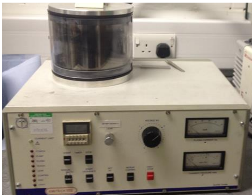
Figure 4-13: A photograph of Bench-top sputter coating system (Emitech SC7640 Sputter Coater, Polaron, UK).
