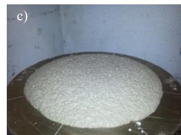
Fig.10. Consistency test for 50%-50% and a) W/S=0.25 , b) W/S=0.35 and c) W/S=0.45 .
