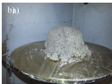
Fig.10. Consistency test for 50%-50% and a) W/S=0.25 , b) W/S=0.35 and c) W/S=0.45 .
