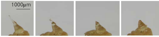
Figure 6. Microneedles removed from porcine skin after a) 0s b) 60s c)120s and d)180s (same scale for all images).
