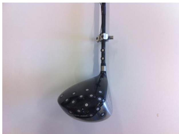
Figure 16 - PONTOS instrumented clubhead
