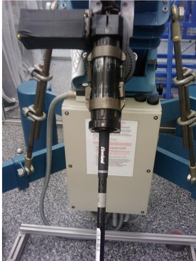
Figure 11 - The current grip on the Miyamae V golf robot
