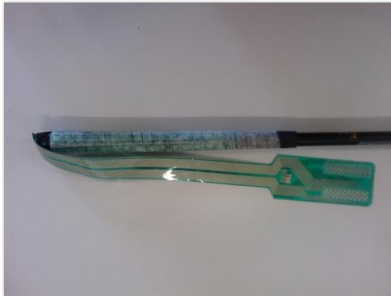
Figure 48 - Tekscan thin film force sensor mounted onto a golf grip
