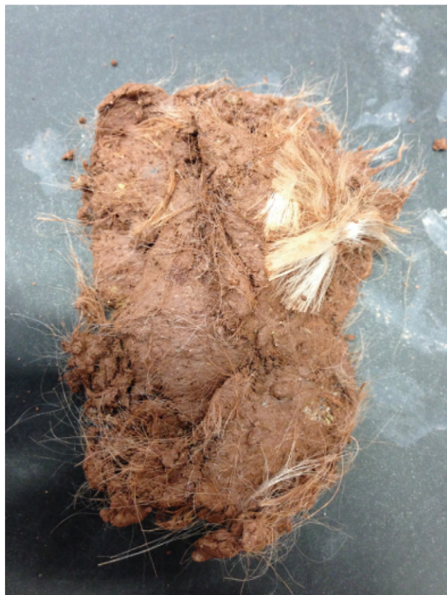
Figure 2. Fibre bunches found within the mix sample at 16% \omega_c (where \omega_c represents moisture/water content)
