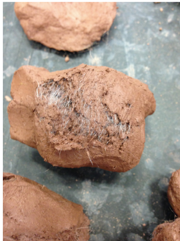
Figure 3. Homogeneous distribution of fibres within the mix sample at 26% \omega_c
