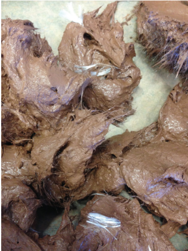
Figure 4. Poor mix quality with a number of fibre bunches remaining in the sample at 34% \omega_c
