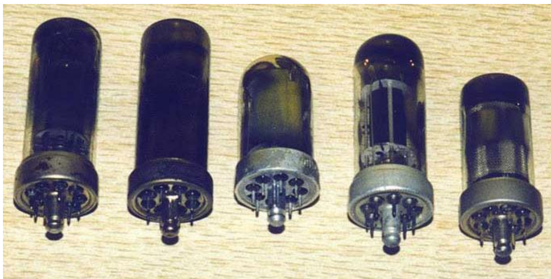
Figure 14- Images Showing Octal Valve Technology
