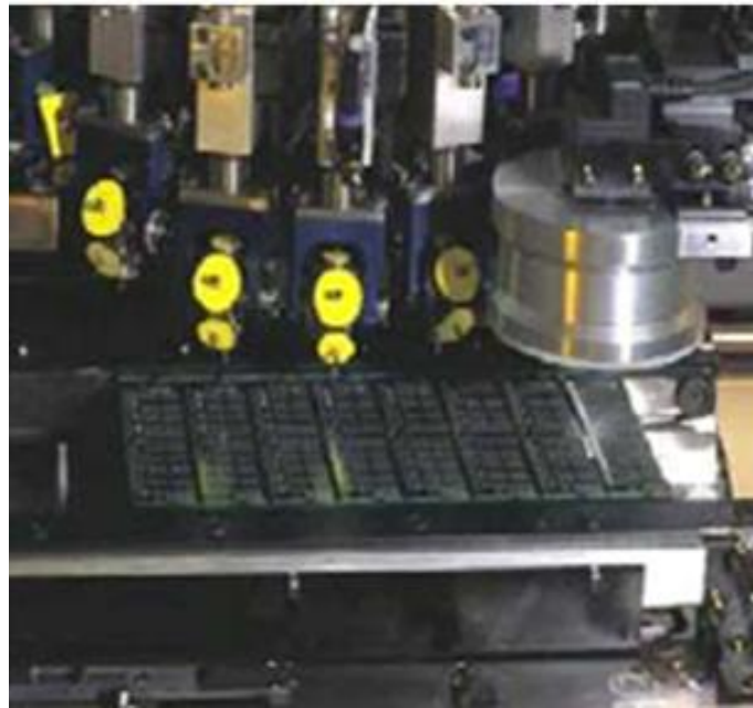
Figure 94 – A Chip-shooter Turret with Twenty Rotary Stations
