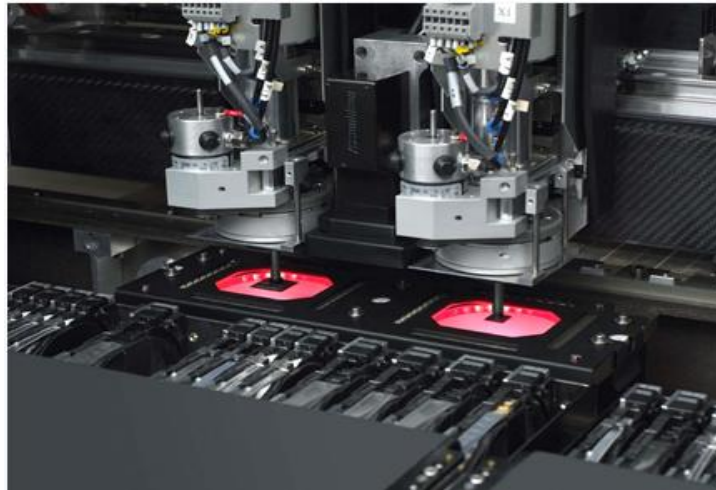
Figure 91 – Dual Head Pick-&-Place Platform with Static Mount Vision Alignment Camera
