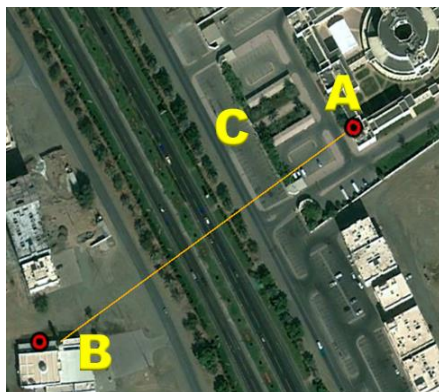
Figure 4.1: Sampling path of the DOAS instrument installed on the premises of Sohar University, Oman; A = light emitter location, B = reflector location and C = car park
