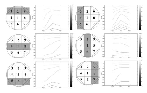
Figure 8: Density gradients for each of the ROIs. Shaded ROIs and correspondent density distribution values for each ROI
