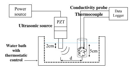
Figure 2: Schematic of the experimental rig
