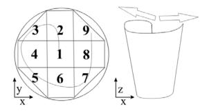
Figure 6: 'Unrolling' methodology for characterization of 3D density distribution
