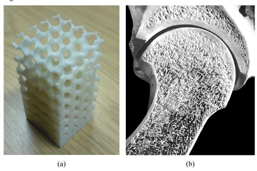
Figure 1: (a) 3D model fabricated by selective laser sintering in polyamide P12 showing the periodic cellular structure; (b) Longitudinal cross section of the human human showing the foam-like structure
