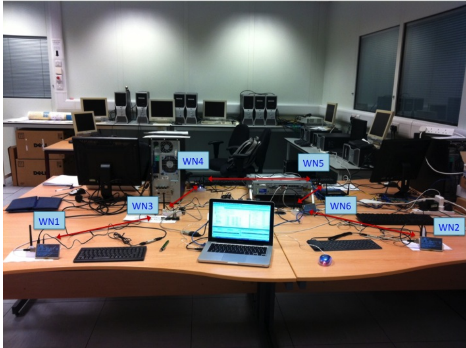
Figure 6.31: Wireless Ad Hoc Network with Six Wireless Nodes
