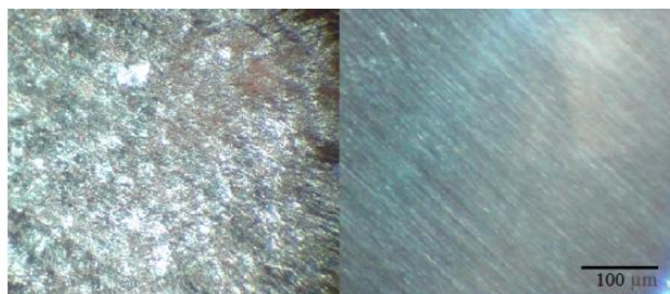
Fig. 1. Optical microscopy images of crucibles used in the DSC experiments. Left: crucible with a rough surface, right: crucible with a smooth surface. The scale bar (100 \mu\text{m} ) is the same the in both images.
