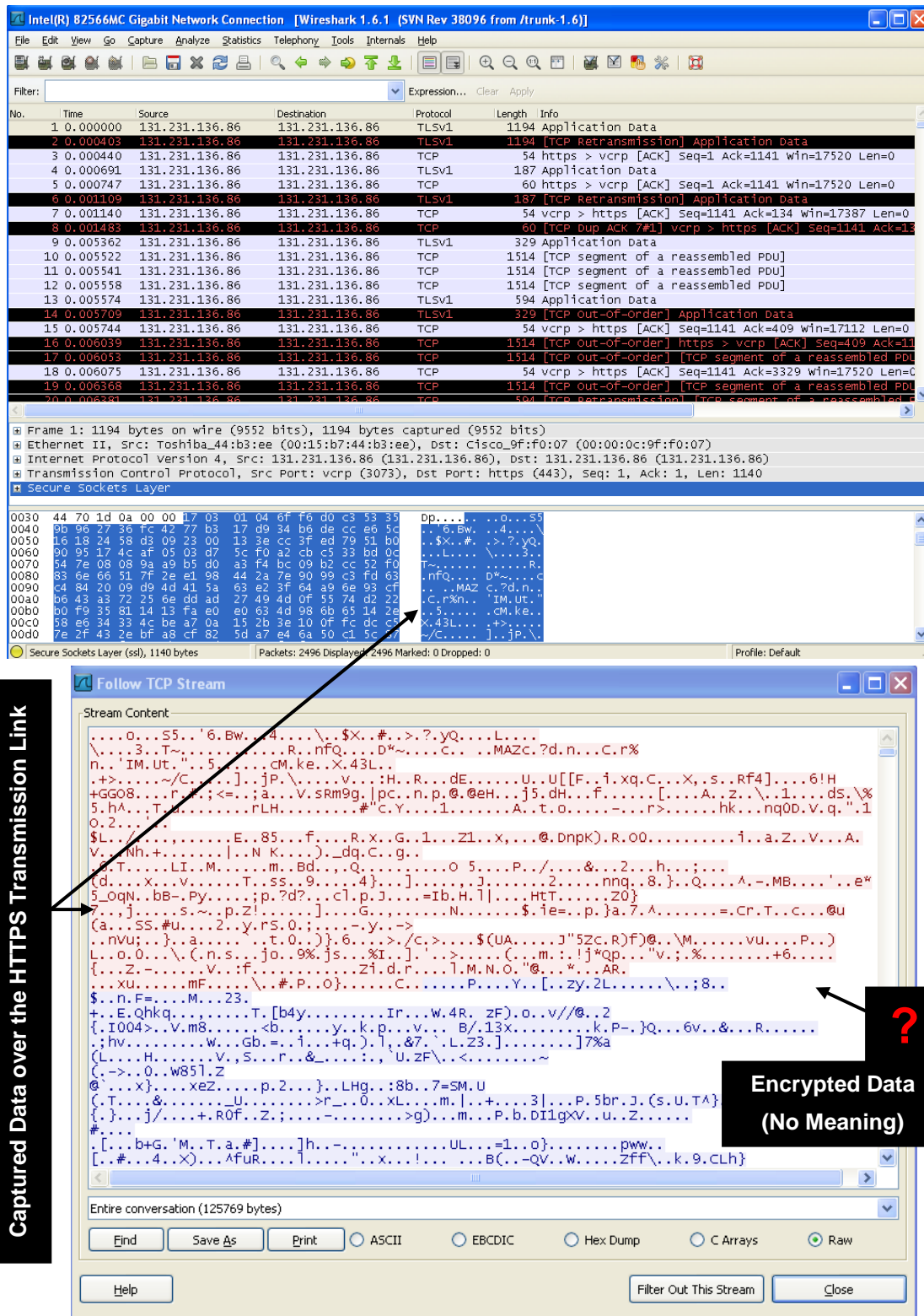
Figure 9-6: Web-HMI Data Encryption Evaluation Using Wireshark Protocol Analyser
