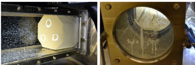
Figure 19. Urea deposits on rear window due to substrate saturation after 10 minutes of dosing at EC5, dosing rate = 2000 g/hr
