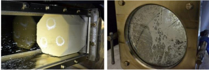
Figure 18. Urea deposits on rear window due to substrate saturation after 10 minutes of dosing at EC2, dosing rate = 1500 g/hr
