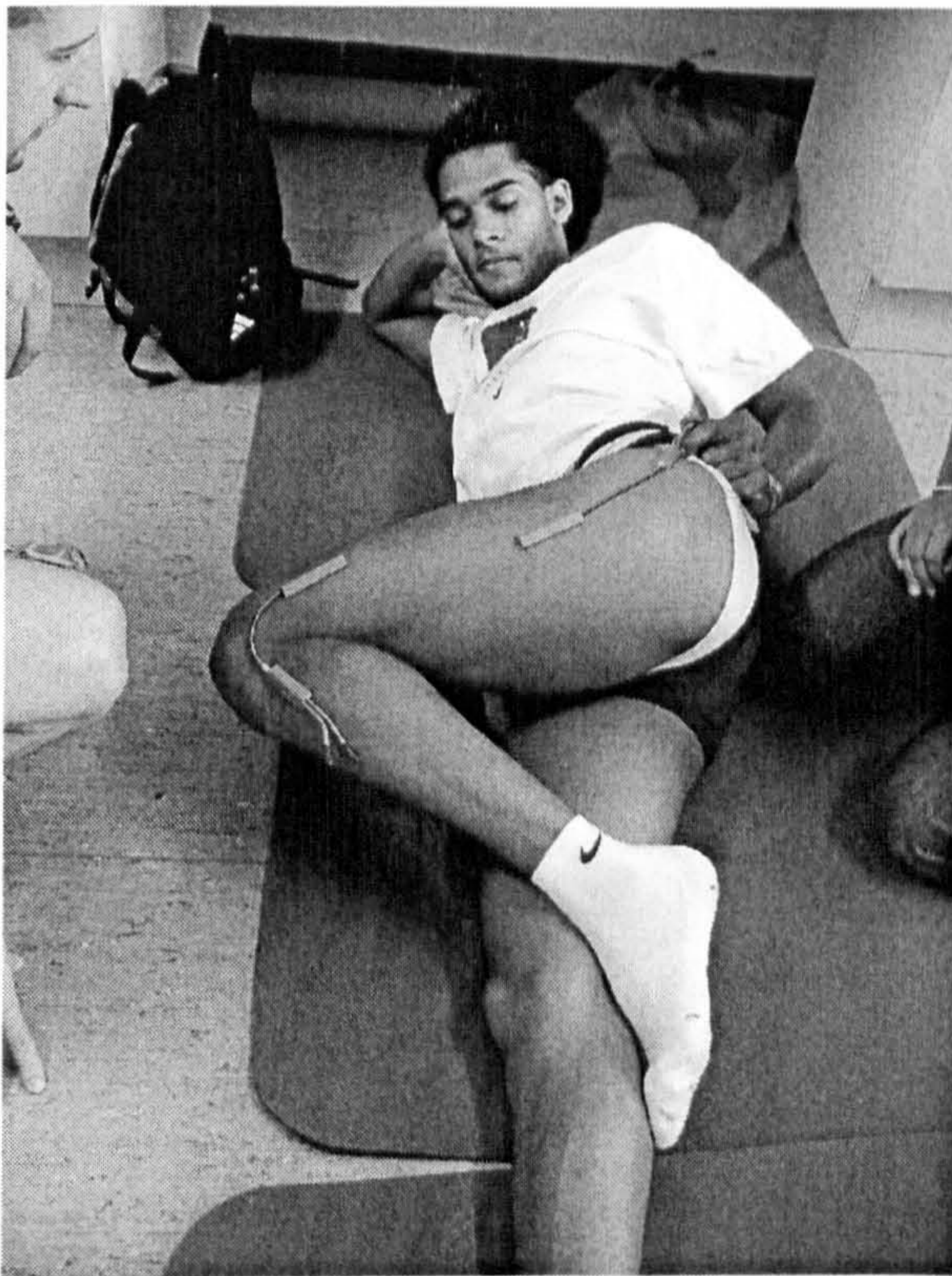
Figure 6.6. Position of the goniometers at the knee and hip joints.
