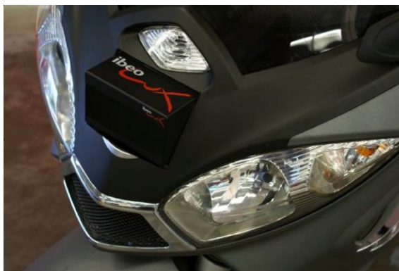
Figure 5: Integration of the Ibeo Lux Laserscanner
