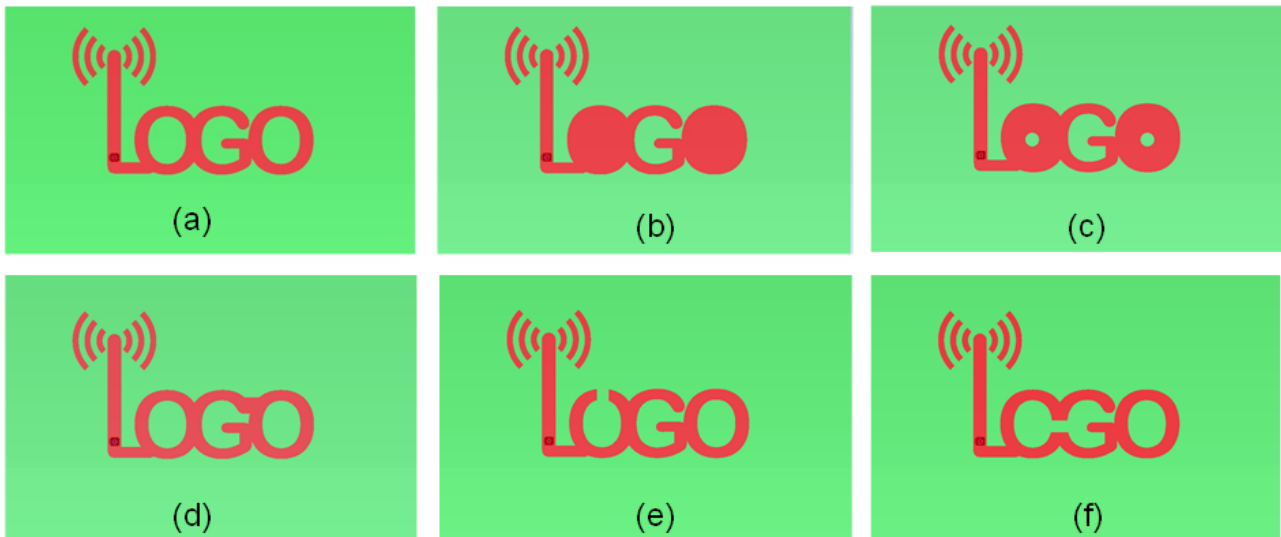
Figure 13. 'Logo' antenna shape variants: (a) original design; (b) solid O's; (c) small holes in O's; (d) G connected to 2 nd O; (e) slot in first O; (f) slot between first O and G
