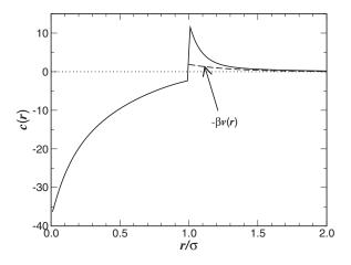
FIG. 19. The direct pair correlation function c(r) obtained from the PY theory for the parameters A=0.55 and  $\epsilon^{-1}=0.41$  and density  $\rho\sigma^3=0.220$ . The dashed line is a plot of  $-\beta v(r)$ . For the corresponding g(r), see Fig. 15, and for the corresponding S(k), see Fig. 17.
