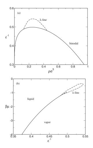
FIG. 11. Phase diagram for  $z_1=2$ ,  $z_2=1$ , and A=0.55, obtained from the RPA DFT theory of Ref. [32]. The solid line is the binodal and the dashed line is the  $\lambda$  line. (a) Plotted in the density  $\rho$  versus  $\epsilon^{-1}$  plane, (b) plotted in the chemical potential  $\mu$  versus  $\epsilon^{-1}$  plane.
