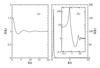
FIG. 17. The static structure factor, S(k), obtained for the PY theory for the state points A=0.55,  $\epsilon^{-1}=0.41$  and for densities (a)  $\rho\sigma^3=0.024$ , (b)  $\rho\sigma^3=0.220$ . For both of these state points the agreement between the PY results and the MC simulations for g(r) is good—see Fig. 15. The inset to (b), shows S(k) on a logarithmic scale.
