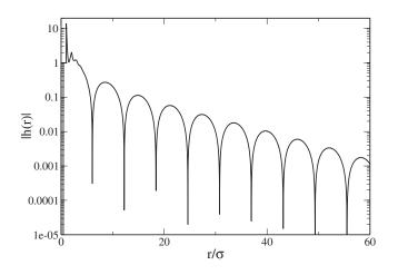
FIG. 16. The modulus of the correlation function h(r) obtained from the PY theory for  $\epsilon^{-1}=0.41$  and  $\rho\sigma^3=0.220$ .
