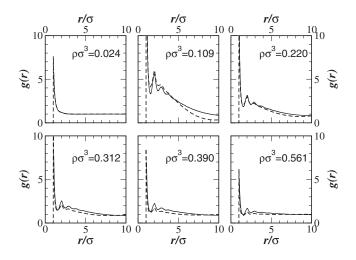
FIG. 15. The radial distribution function, g(r), obtained from simulation (solid lines) and the PY theory (dashed lines) for  $\epsilon^{-1}$  =0.41 at the particular selection of densities indicated. Note that in both the simulations and theory, a jump discontinuity occurs in g(r) between  $\rho\sigma^3$ =0.024 and  $\rho\sigma^3$ =0.109. Within the PY theory, this jump occurs at  $\rho\sigma^3$ =0.04.
