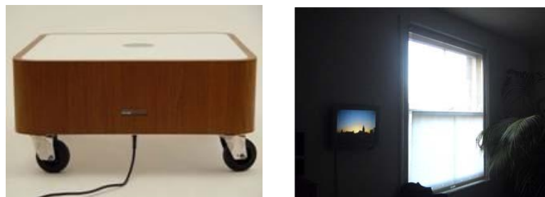
Fig. 30 / 31. Equator Project. 'Key Table' and 'Drift Table' are conceptual designs that rely on sensing the weight of objects placed on surfaces, reflecting people's activities at home (2000-2002). Equator Project - Video Window (on the right), 2000-2002.
