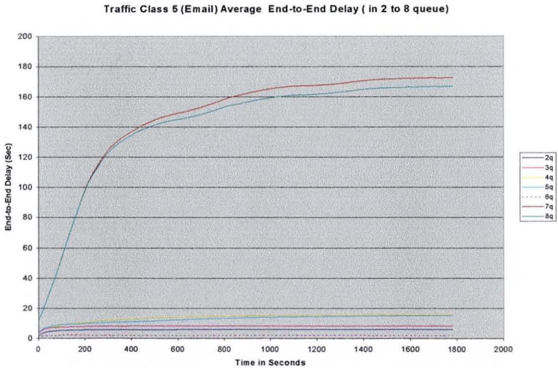
Figure 6.6: Showing end-to-end delay for traffic class 5, in 7 simulation scenarios with each scenario employing different number of queues varying from 2- queues up to 8-queues. Identical input traffic parameters used in all the seven scenarios.
