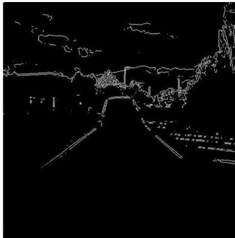
Figure 3-3: Sample image with Sobel filter applied
