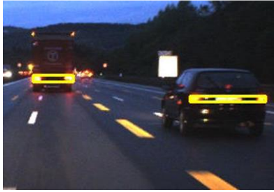
Figure 2-3: Rear light detection Source: Schamm et al. (2010)
