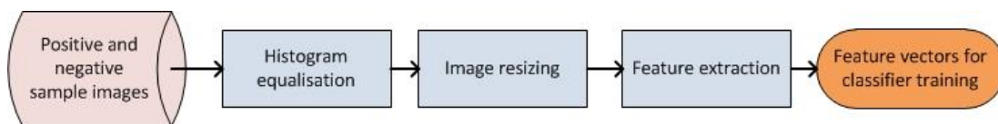
Figure 3-15: Image feature extraction process
