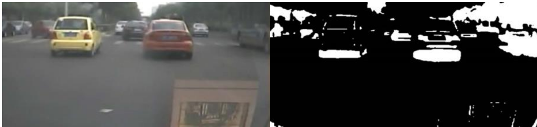
Figure 2-1: Original image (a), shadow segmentation (b). Source: Li and Guo (2013)
