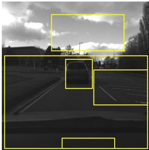
Figure 3-14: Bounding boxes after small object removal
