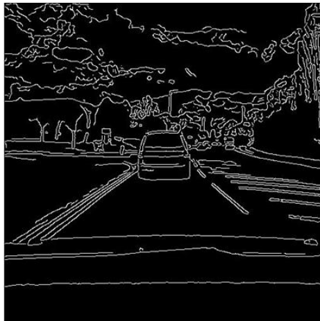
Figure 3-4: Sample image with Canny filter applied
