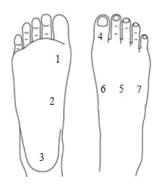
**Figure 1 Anatomical positioning of thermocouples on the right foot.** Site codes: 1-plantar ball; 2-plantar arch; 3- plantar heel; 4-base of toe 1; 5- central dorsal; 6-medial dorsal; 7-lateral dorsal.
