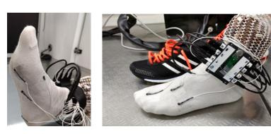
Figure 2 Positioning of temperature and relative humidity sensors on the right foot.
